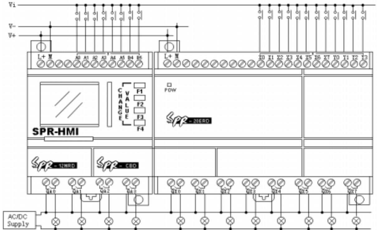
Fig6.9 SR-20ERD connected to SR-12MRDC
