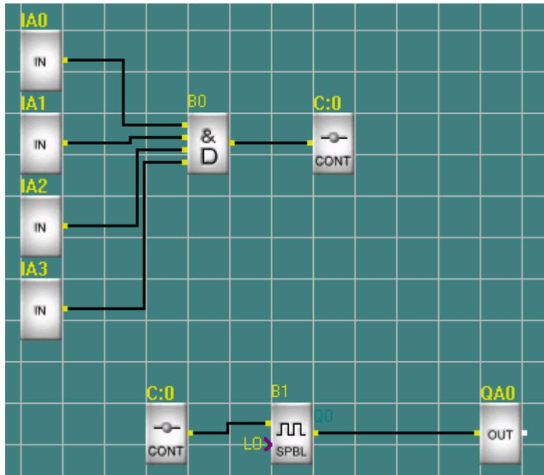
**Notes:** In this program, C0 is the two connection points of the wire, that is to say that, the output of B0 is connected to input of B1.
