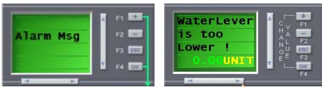
When IA1 become 1 status, then the LCD will display the alarm message and indicate the water lever value.
