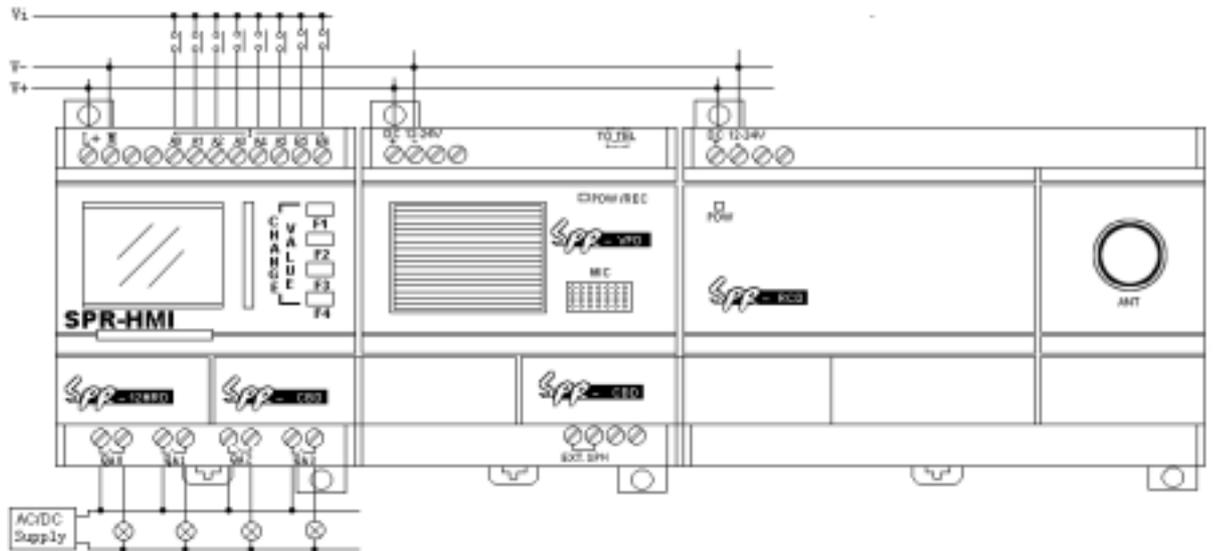
Fig6.3 SR-RCD connected to SR-12MRDC and SR-VPD
