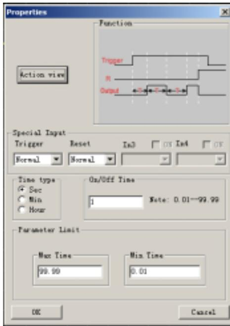
Fig. 3 . 15 Module with the timer Property Setup
