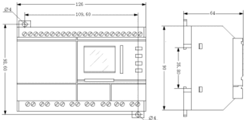
**Fig. 2.3 Installation Dimension of SR-22 Series (MM)**
