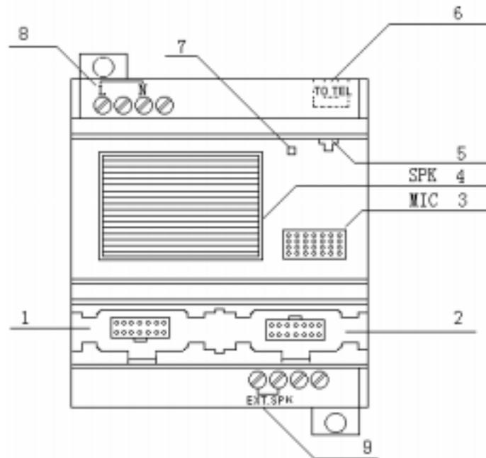
Fig. 5.1 Structure of SR-VP Series Voice Module
