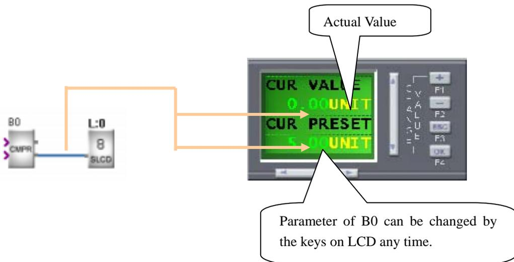
**Fig. 4.4 Actual Value & Parameter of the Running**
