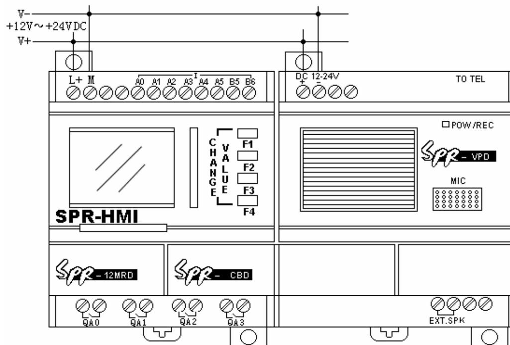
Fig. 5.3 Connection between SR-12MRDC and SR-VPD
