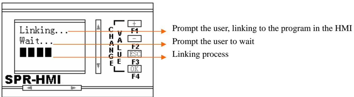
**Fig. 10.18 Process Interface of Linking to HMI**
