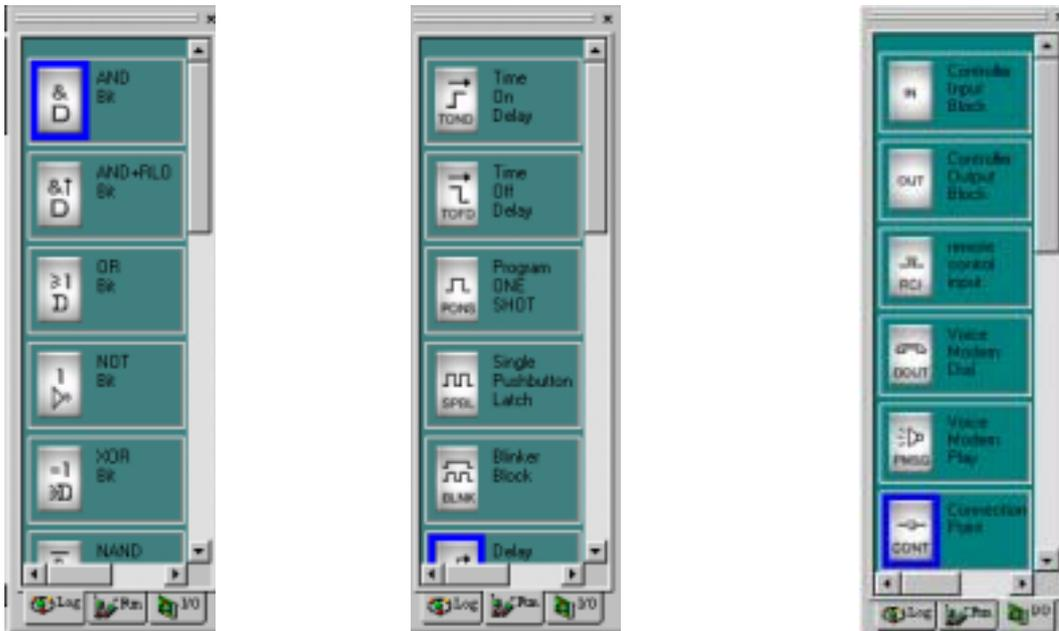
Fig4.5 ( a )Basic Module      Fig4.5 ( b )Special Module      Fig4.5 ( c )Input/output Module
