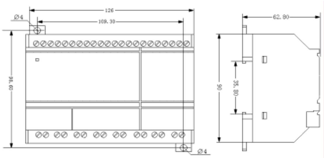
**Fig. 2.5 Installation Dimensions of SR-20 and SR-RC Series (MM)**
