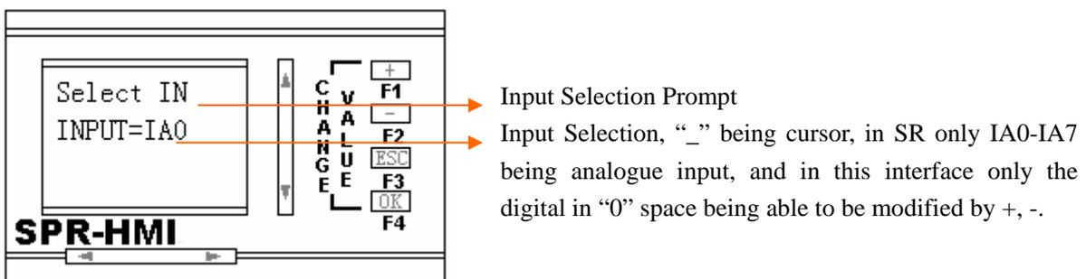
**Fig. 10.25 Selection Interface of A B Value Demarcating Input**
