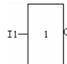
This function block is called as NOT, because if the input status is 0, then output Q is 1, and vice versa. In other words, NOT is the phase inverter for the input point.
