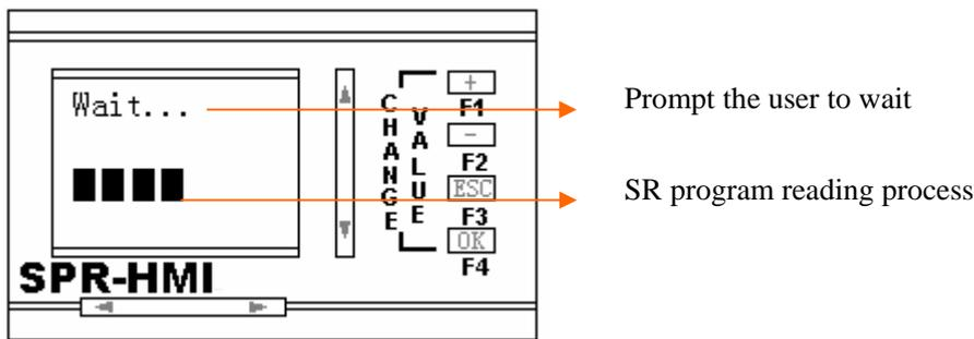
Fig. 10.21 Reading Process Interface
