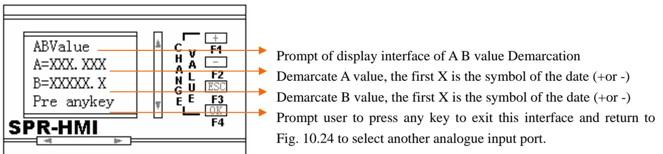
**Fig. 10.28 Input Interface of A B Value Demarcating Input**
