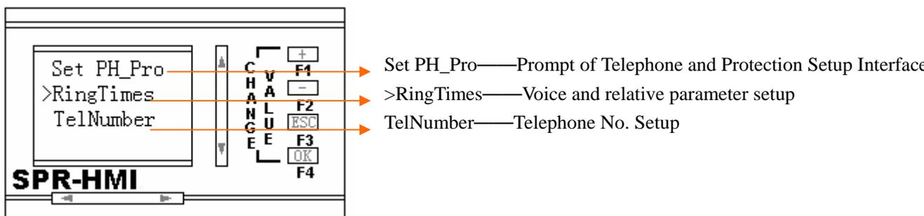
**Fig. 10.35 Telephone Setup and Protection Interface**
