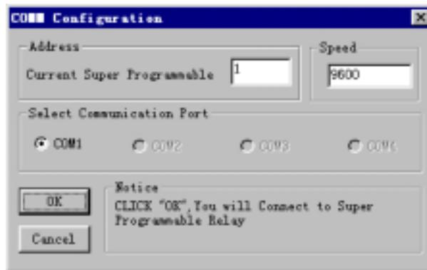
Fig 4.17 Set Up Port and Baud Rate
