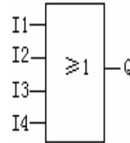
This function block is called as OR, because the status for at least one of the inputs I1, I2, I3 or I4 is 1 (i.e. closed), then output Q is 1.
