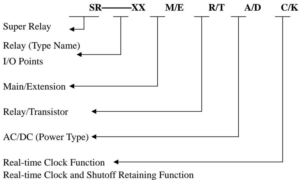
**Note:** M means main machine, E means extension module
