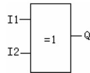
When the statuses of all the inputs are not the same, the output status of XOR is 1. When the statuses of all the inputs are the same, the output status of XOR is 0.
