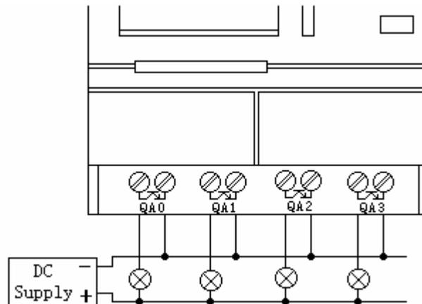
**Fig. 2.12 Transistor Output**
