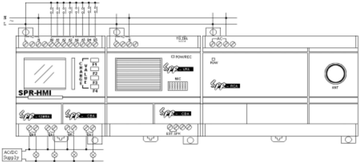
Fig6.2 SR-RCA connected to SR-12MRA and SR-VPA
