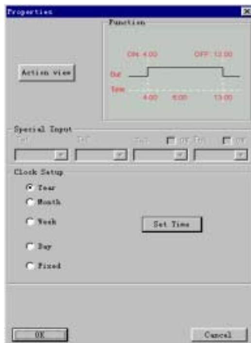
Fig. 3 . 19 Setting CW Clock Switch Block Properties
