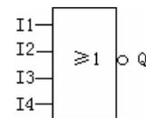
In NOR function block, when the statuses of all the inputs are low potential (status 0), then the output is connected (status 1). If the status of any input is high potential (status 1), then the output is opened (status 0).
