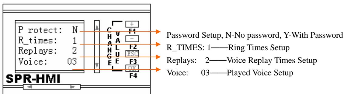
**Fig. 10.36 Voice and Relative Parameter Setup Interface**
