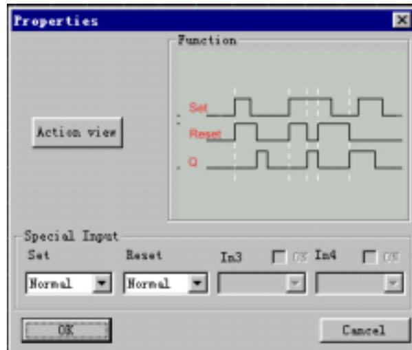
Fig. 3.18 Setting Properties for RS Relay
