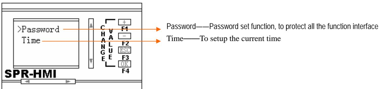
Fig. 10.22 Time and Password Setup Interface
