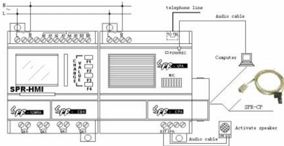
Fig. 5.22 Wiring Diagram of Voice Module Recording
