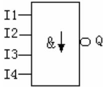
Only when the status of at least one of the input is 0 and statuses of all the inputs in the last period are 1, the output status of this NAND with RLO borderline test is 1.
